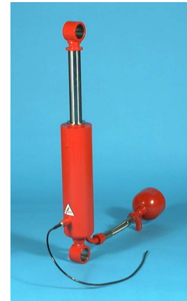
Semi-active heavy vehicle damper (supplied by Koni) used to improve the ride further over the optimum passive case.
