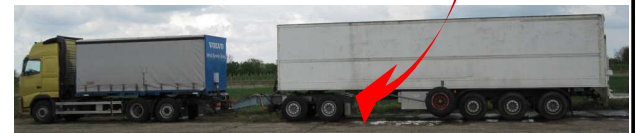
Figure 6: Actively steered (7 of 8 axles) EMS combination with Truck-Dolly-Semitrailer. Dolly demounted from link trailer
