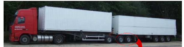
Figure 5: Active steered (6 of 7 axles) B-double vehicle combination. Rear of link trailer demountable to form dolly
