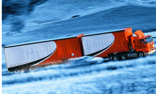
Figure 1: Double-trailer vehicles (B-Doubles and A-Doubles) are used widely in Australia, New Zealand, South Africa, Canada and the USA.
